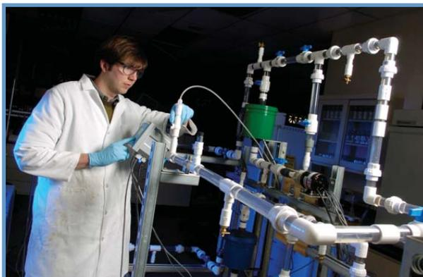
Experimental pipe loop system for evaluation of real times chlorine sensors. Dr. Damian Helbling is adjusting the sensor calibration. (Photo Courtesy Carnegie Mellon University)
